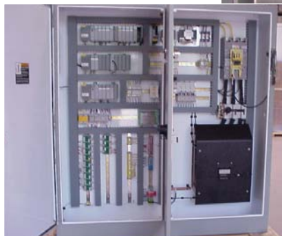
Custom clutch/brake control cabinet
